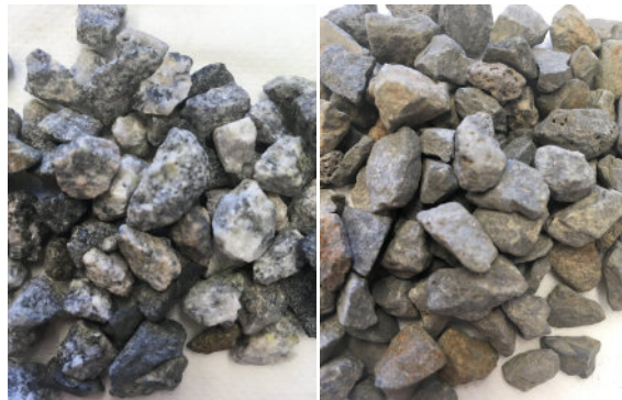
Figure 23: Picture of the aggregates used for the experiment, granite on the left and basalt on the right
