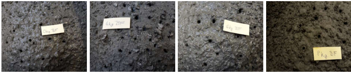
Figure 5. Photo documentation of the surface of test samples with various basalt fibres dose: a) 0 kg, b) 4 kg, c) 6 kg, d) 8 kg.
