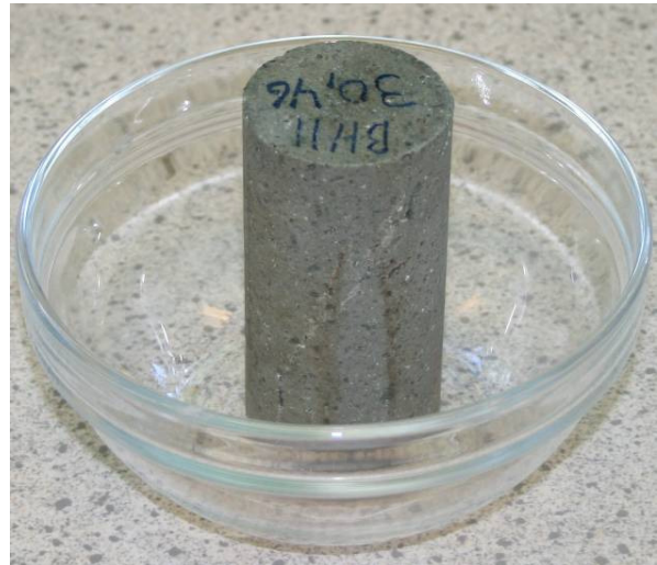
Nr. 23: Rhyolite (homogeneous) Failure at: \sigma_1 = 52,39 MPa and \sigma_3 = 2,00 MPa
