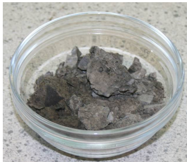
Nr. 39: Conglomerate Failure at: \sigma_1 = 39,40 MPa and \sigma_3 = 2,00 MPa
