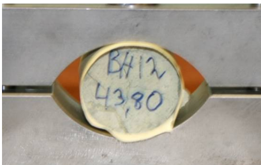
Nr. 80: Rhyolite (inhomogeneous) \sigma_t = 2,12 MPa.
