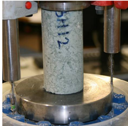
Nr. 30: Rhyolite (inhomogeneous) \sigma_c = 9,0 MPa.
