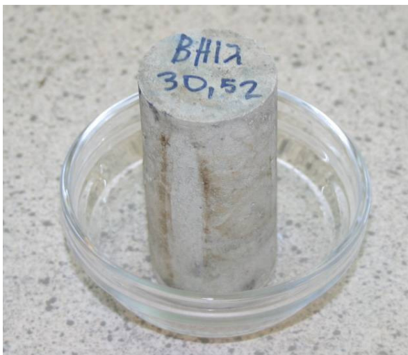
Nr. 33: Rhyolite (inhomogeneous) Failure at: \sigma_1 = 36,04 MPa and \sigma_3 = 2,01 MPa
