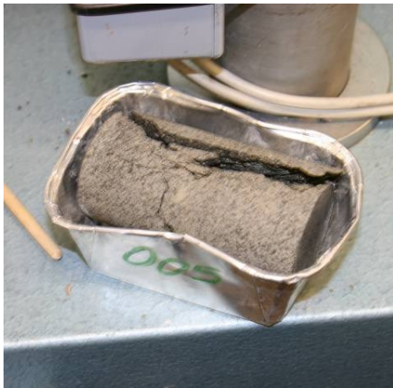
Nr. 10: Altered olivine tholeiite \sigma_c = 65,0 MPa.
