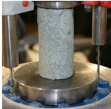
Nr. 32: Rhyolite (inhomogeneous) \sigma_c = 19,0 MPa.
