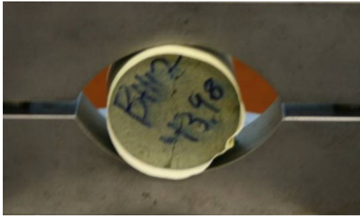
Nr. 82: Rhyolite (inhomogeneous) Test failure.
