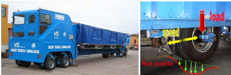
Figure 2.4 The HVS machine operated at VTI in Sweden.
