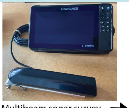
Multibeam sonar survey lake bathymetry and volume (Summers 2023 + 2024)
