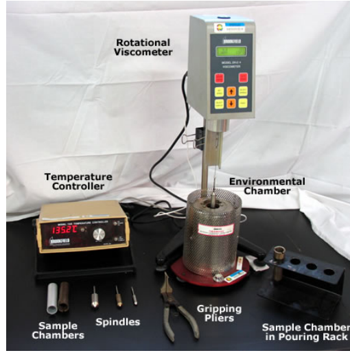
Figure 4.4: The equipment used for the rotational viscosity test [66].
