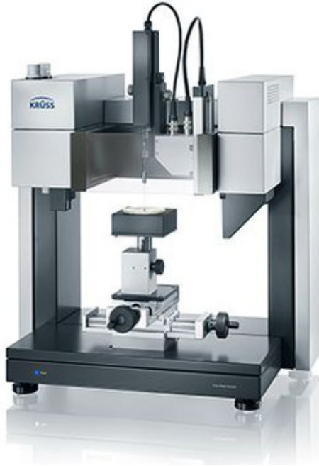
Figure 4.5: A photo of a drop shape analyzer, the equipment used for the sessile drop technique [67].
