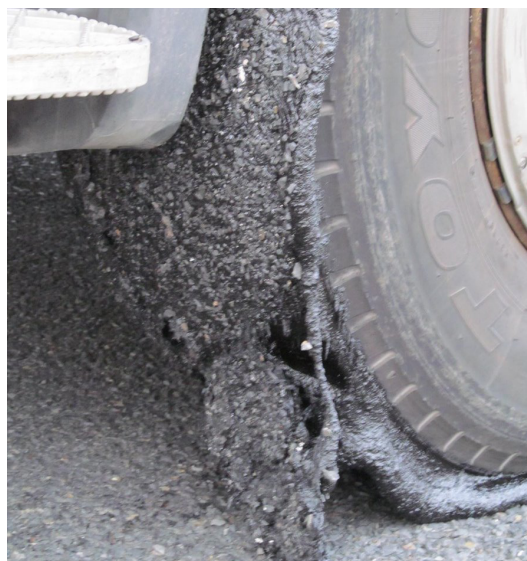
Figure 2.3: A tire that has been driven through an area where severe bleeding has occurred [15, 18].
