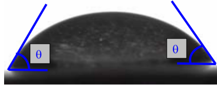
Figure 4.7: An image of a drop captured by the camera on the drop shape analyzer [2].
