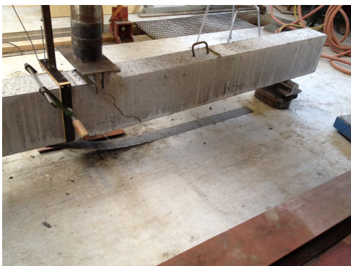
Figure 5-25. Crack pattern for BFc9 (EPOXY1), de-bonding failure.
