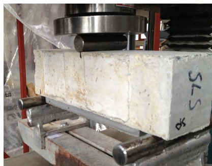
Figure 4-25. Flexural testing on small-scale beam specimens.
