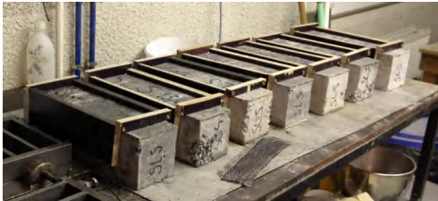
Figure 4-23. Testing cement-based material on small beams.
