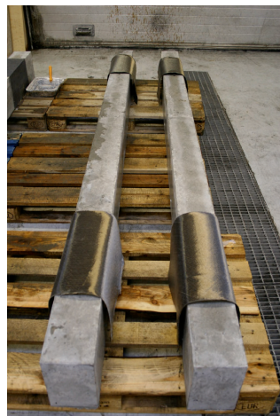
Figure 4-12. BFRP sheet application.
