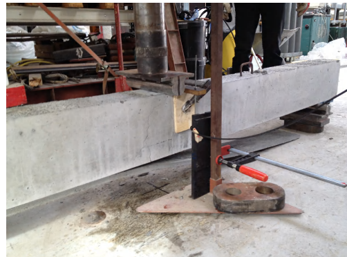
Figure 5-20. BFc4 (AK2), bonding failure during testing.
