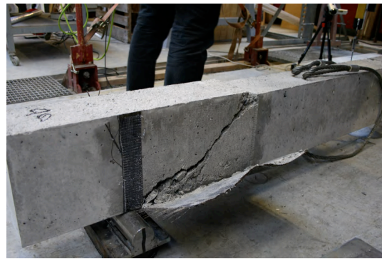
Figure 5-4. Crack pattern for BSa3 at ultimate load.
