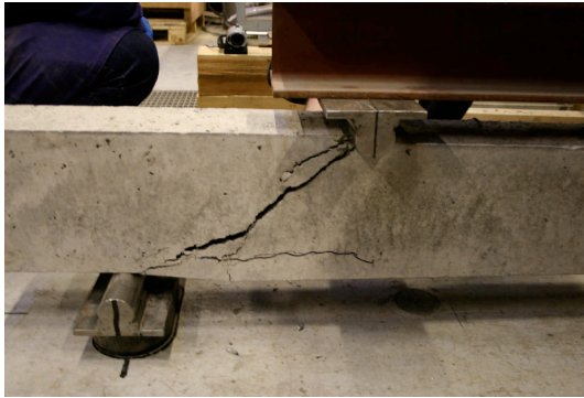
Figure 5-1. Crack pattern for BSa1 at ultimate load.
