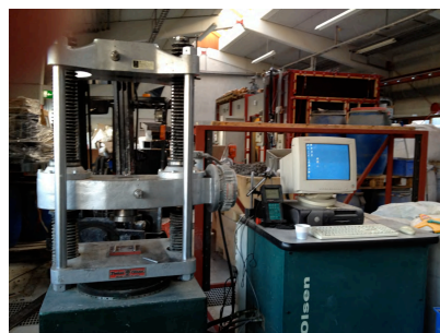
Figure 4-18. TinusOlsen testing machine.
