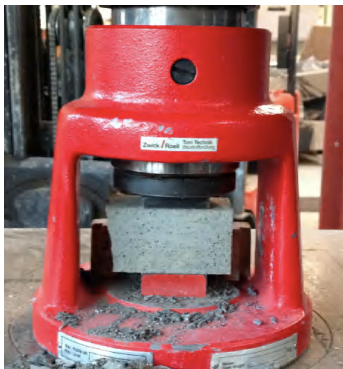
Figure 4-22. Compressive strength test, before testing.
