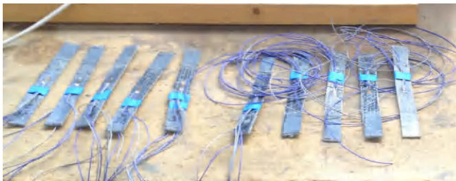
Figure 4-26. Tensile test specimens.
