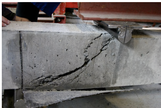
Figure 5-5. Crack pattern for BSa4 at ultimate load.
