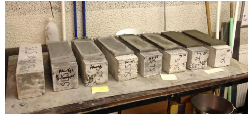
Figure 4-24. Testing cement-based material on small beams,
