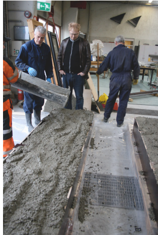
Figure 4-9. Casting of beams specimens.
