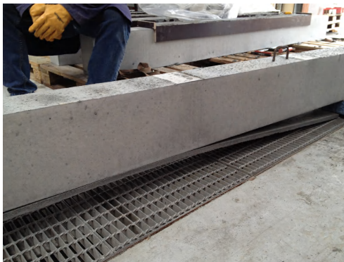
Figure 5-19. BFc3 (AK1), Bonding failure before testing.
