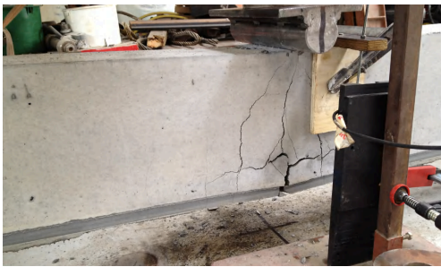
Figure 5-23. Crack pattern for BFc6 (Fibre2).
