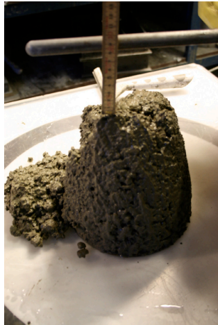
Figure 4-6. Slump test, C25.
