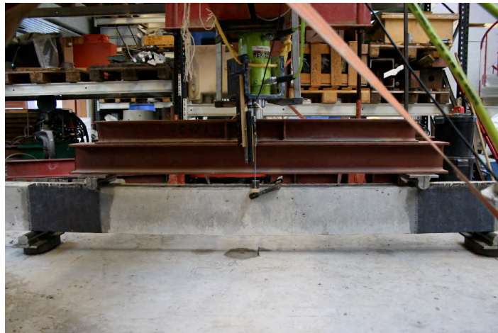
Figure 4-15. Four-point load test.
