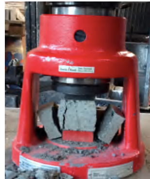
Figure 4-21. Compressive strength test, after testing.
