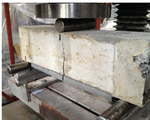
Figure 5-28. Crack pattern for small-scale beam
