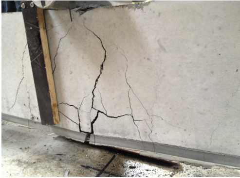
Figure 5-21. Crack pattern for BFc5 (Fibre1), fully composite action between concrete and CBM.
