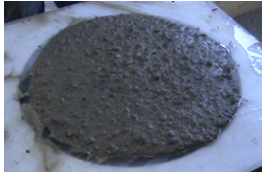
Figure 4-7. Slump flow test, C35 (SCC).
