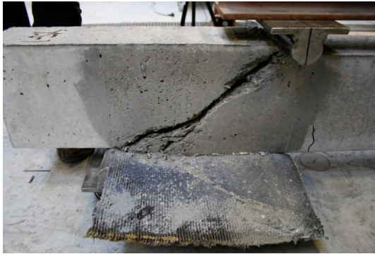
Figure 5-7. Crack pattern for BSa5 at ultimate load.
