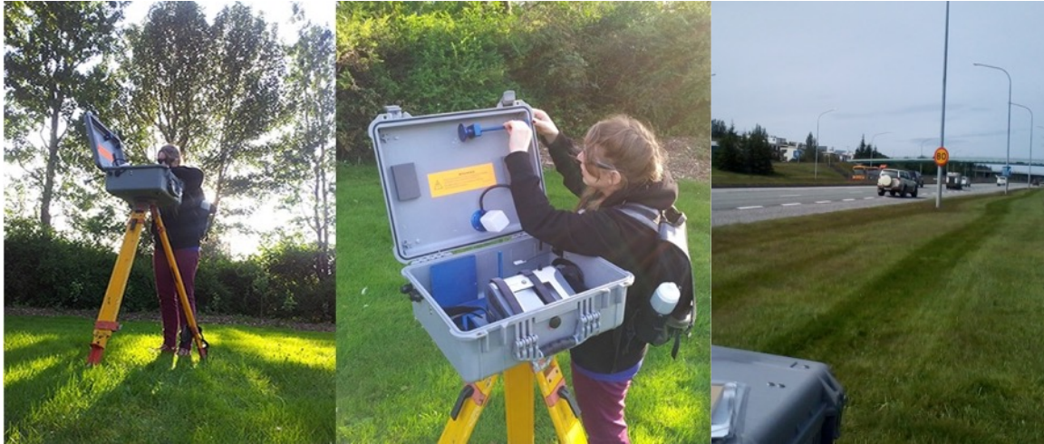
Figure 5.1 Setting up a TSI Optical Particle Sizer, Model 3330 at the Klambratún location, behind vegetation barrier (left and middle); Average traffic conditions on Location 1 (right).
