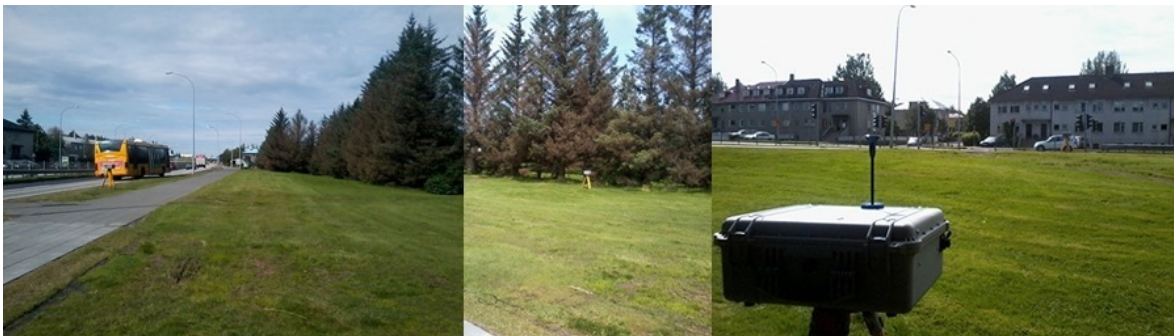
Figure 5.9 Klambratún location without the barrier with one instrument placed next to the road, and the other placed ~25 m behind it, perpendicular to the road with no barrier between them.
