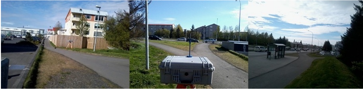
Figure 5.6 Location close to the 365 Media building on the Miklabraut road, Reykjavik, Iceland showing a device placed next to the road, and a device placed on a path perpendicular to the road and directly exposed to it.
