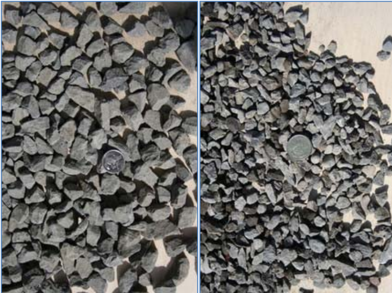
Figure 24 - 11-16mm chips (left) and 8-11mm (right) used on the job
