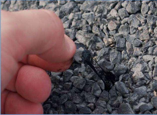
Figure 40 - The chips had good embedment and the binder elasticity was intact
