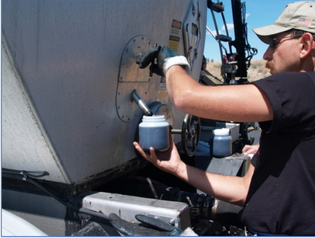
Figure 10 - Taking sample from the asphalt hauling truck
